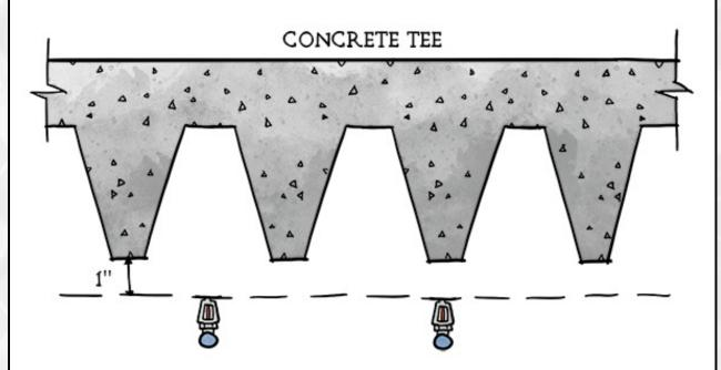
SPRINKLERS ARE PERMITTED AT OR ABOVE A HORIZONTAL PLANE 1" BELOW BOTTOM OF STEM (IF ABOVE BOTTOM) COMPLY WITH BEAM RULE
